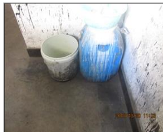
Photo of non-conformity NC no secondary container for glue.JPG
